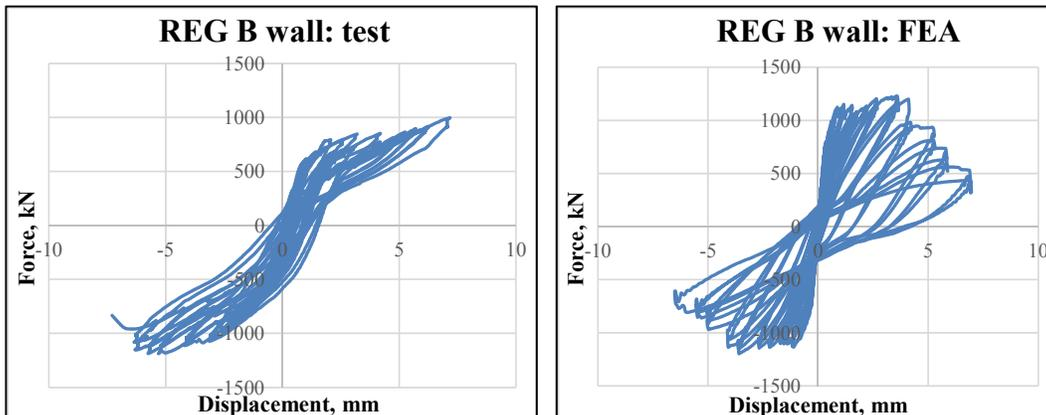
Figure 6. Lateral Force vs. Displacement Curve for REG B wall (after 975 days of accelerated aging)
