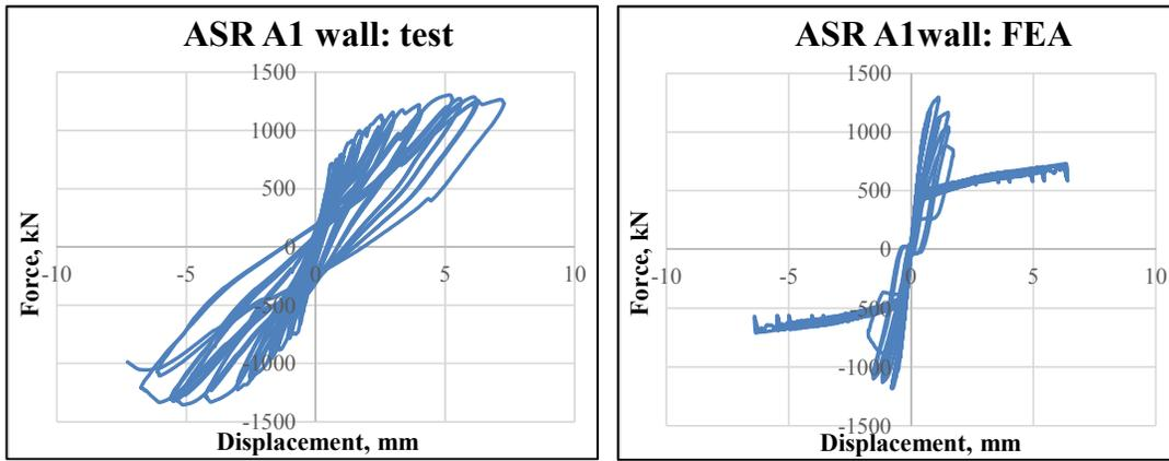
Figure 7. Lateral Force vs. Displacement Curve for ASR A1 wall (after 260 days of accelerated aging)
