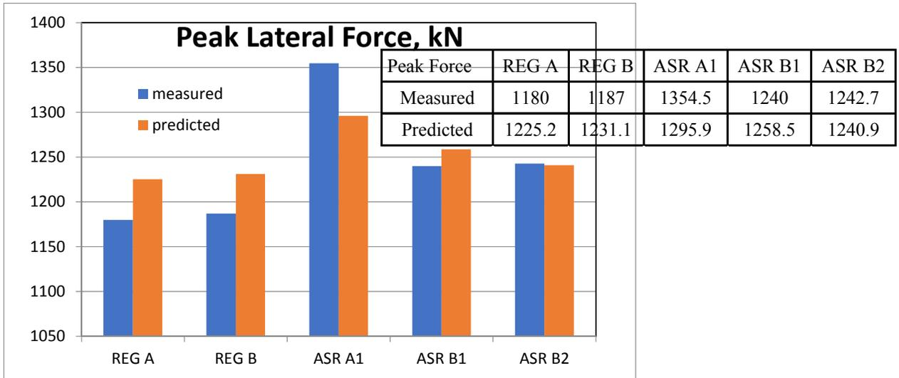
Figure 4. Predicted and measured Maximum Shear Capacity for all Walls
