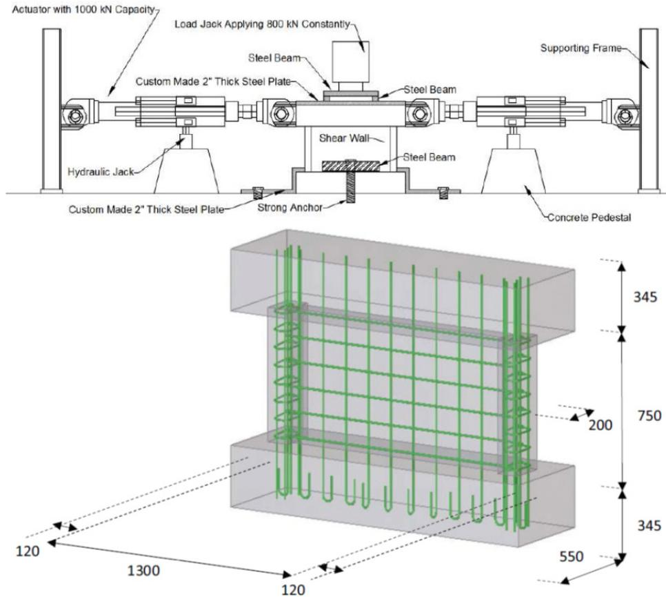
Figure 1. Test setup [4] and wall geometry. All dimensions are in cm [6]
