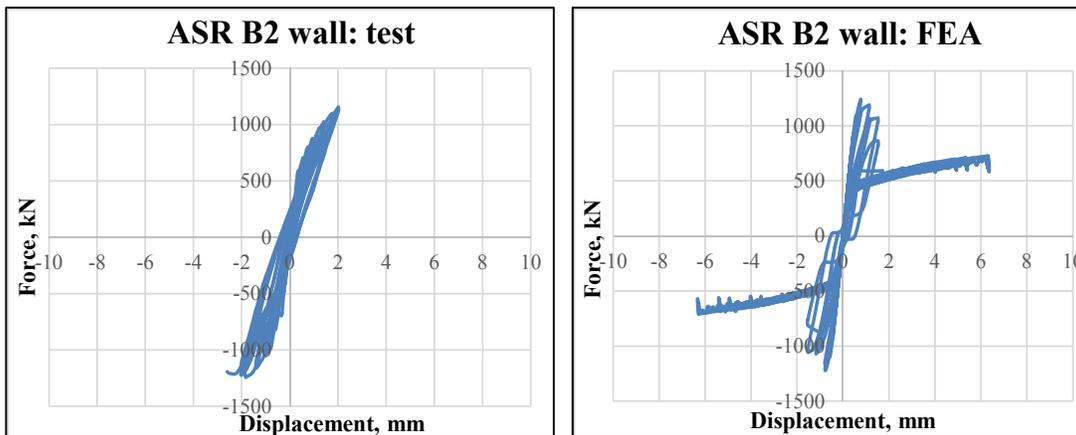
Figure 9. Lateral Force vs. Displacement Curve for ASR B2 wall (after 995 days of accelerated aging)
