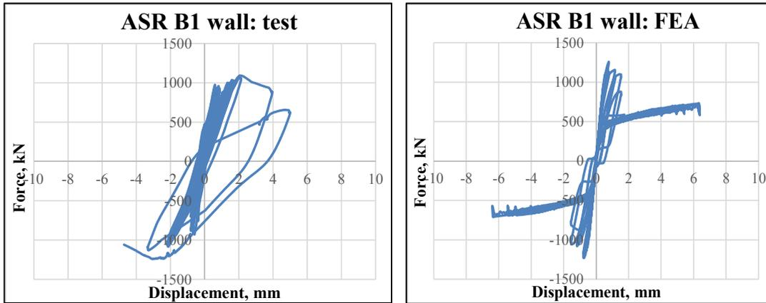
Figure 8. Lateral Force vs. Displacement Curve for ASR B1 wall (after 610 days of accelerated aging)
