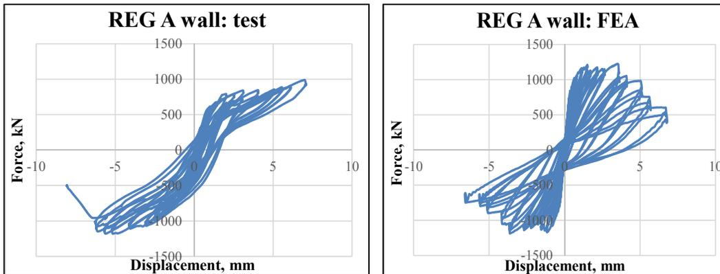
Figure 5. Lateral Force vs. Displacement Curve for REG A wall (after 240 days of accelerated aging)
